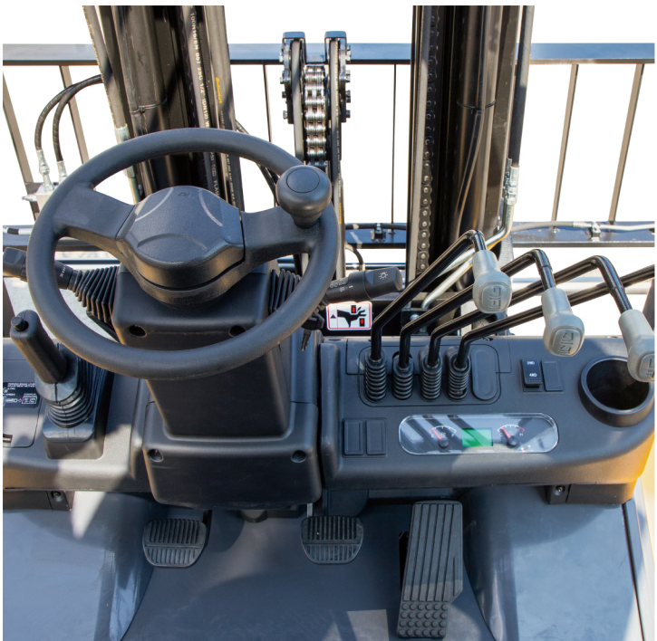
Ergonomic instrument panel: integrated handle switch, ratchet type hand brake and integrated electro-hydraulic reversing handle
