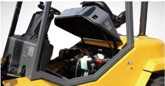
High angle hood open for easy maintenance
