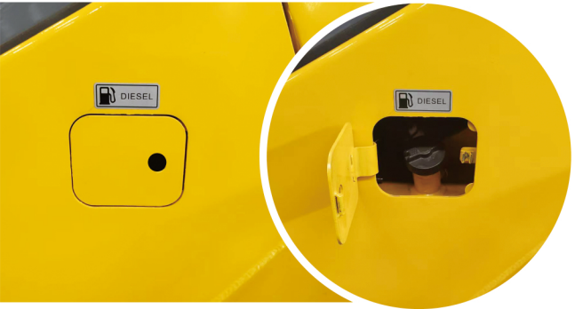
The concealed refueling port, effectively avoids the intrusion of rainwater and sediment
