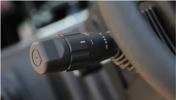
Ergonomic instrument panel: integrated handle switch, ratchet type hand brake and integrated electro-hydraulic reversing handle
